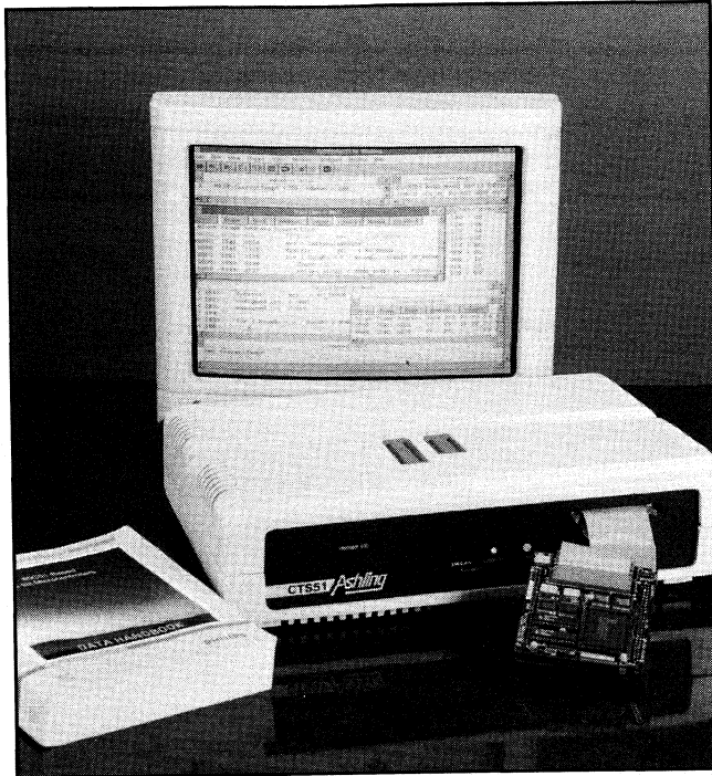
Ashling's CTS51 Universal Microprocessor Development System for Philips Microcontrollers
